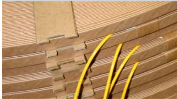
Figure 3 – Picture of fiber optic sensors
