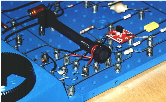
This picture shows the RF part of the receiver. The coil consists of 9 turns which need to be very carefully and closely wound. The red coil is for the antenna and should be immediately adjacent to the main coil. Both coils should be near the end of the ferrite coil. In practice, I never used an antenna. For optimal contact the transistor is mounted *upon* the components (as is suggested by the Philips manual for the EE2010/13 FM receiver). This is good practice for all designs.
