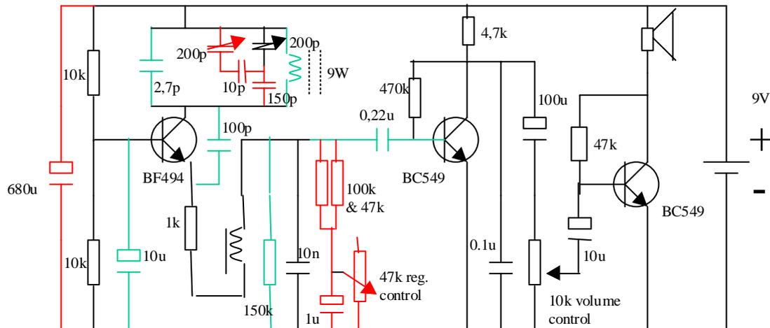
The figure above shows a schematic diagram of the receiver. A red color denotes a newly added component, a green one indicates a change of value for an existing component. The latter has been done to allow the three shortwave broadcast bands to be in the tuning range without the need for bandswitching. The extra components can be easily added to the original construction diagram in the EE2003 manual.
