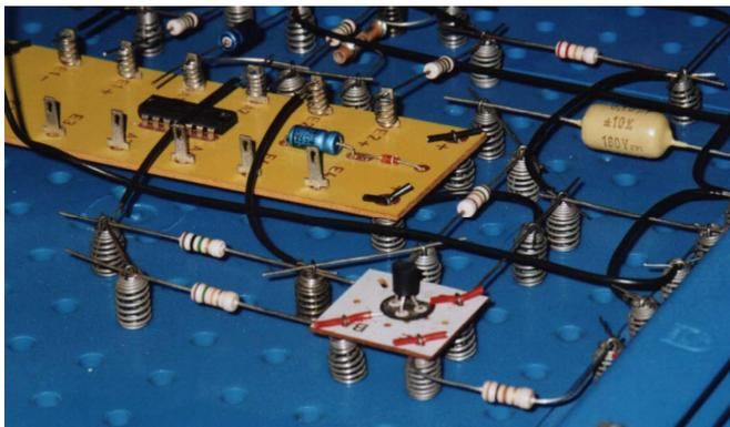
The LF part of the receiver is shown here. It appeared to be good practice to always mount the transistors and ICs upon the components and wires, since this provides for much better contact. Isolated wire is used to fix them. In this way you can even walk around with your receiver without hearing any disturbances.
