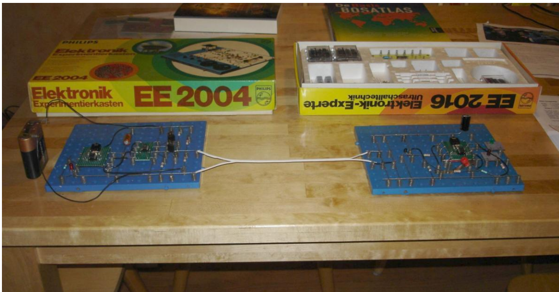
Figure 8: Test bench configuration with a short network wire. In the final successful test the network wire length was 20m.
